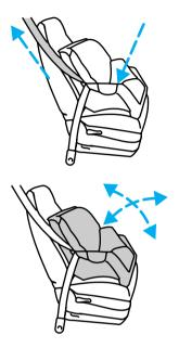
10. Try to pull the belt out of the retractor to make sure the retractor is in the automatic locking mode (you should not be able to pull more belt out). If the retractor is not locked, unbuckle the belt and repeat steps two through nine.
